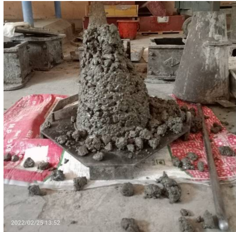
Fig. 3 Slump cone test
