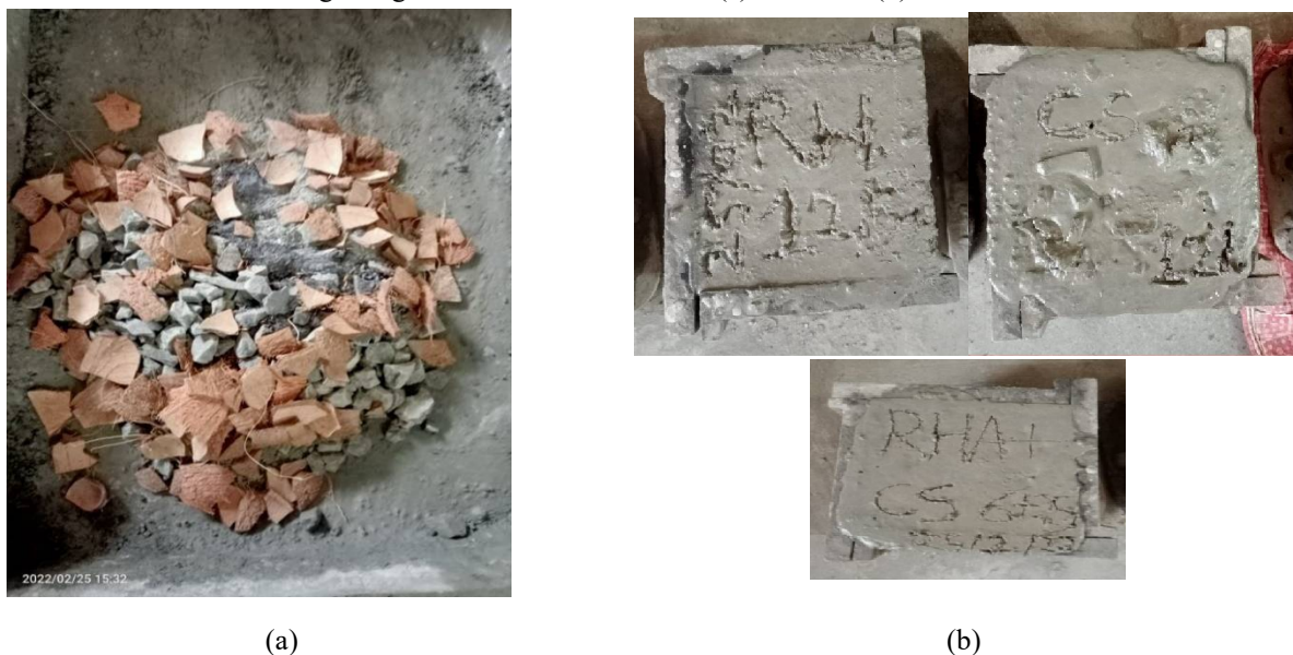
Fig. 2 Blocks preparation (a) Dry quantities of material for 12.5% CS, 9% RHA in concrete (b) Sample Photos of blocks
