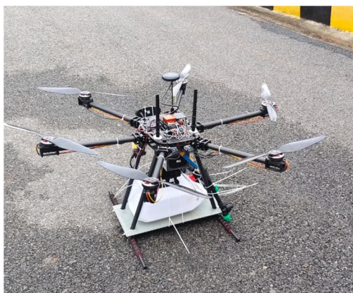
Fig2: Hexacopter drone with Spray system
