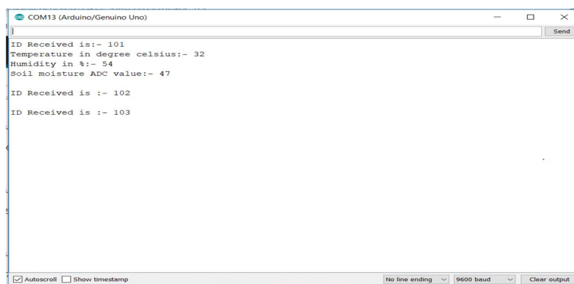
Fig.8 Slave 1 node output at serial terminal
