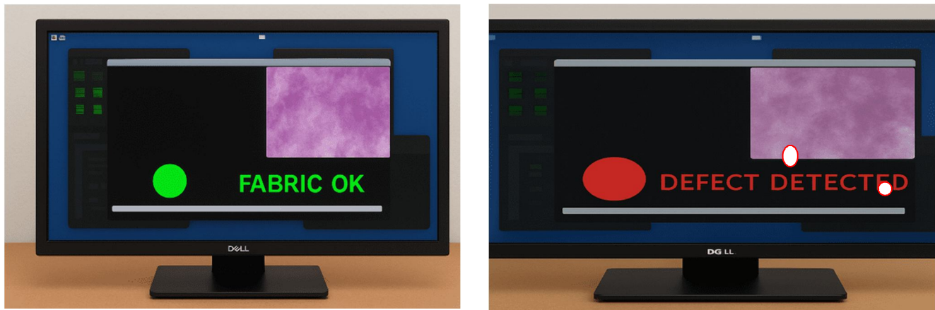
Fig. 12 Graphical User Interface for Machine Control and Defect Tracking with Live Camera Feed and Instant Alert Notifications
