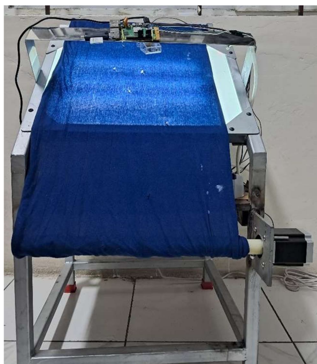
FIG. 12 FINAL PROTOTYPE SETUP OF THE AI-BASED FABRIC DEFECT DETECTION SYSTEM
