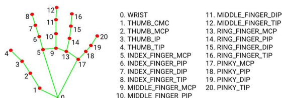
Fig. 1. Hand landmark detection using MediaPipe for sign language recognition
