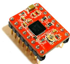
Fig 8: A4988 Stepper Motor Driver
