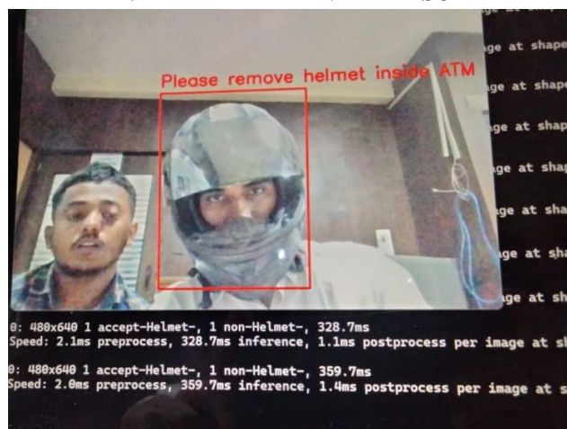
Fig. 3. Detected a person wearing helmet inside the ATM premises.
