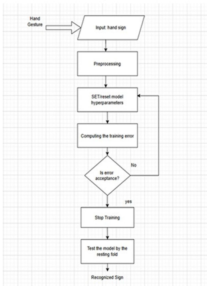
Fig. 1. System Architecture of the proposed AI Hand Sign Detection and Recognition System.
