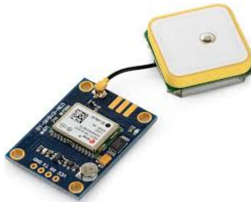
Fig. 2: NEO-6M GPS Module for Real-Time Location Tracking
