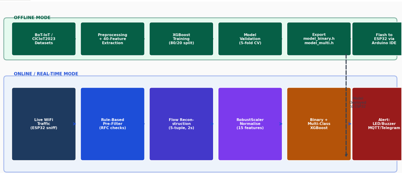
Fig. 2 Dual-mode pipeline: offline training and validation feeding live ESP32 deployment
