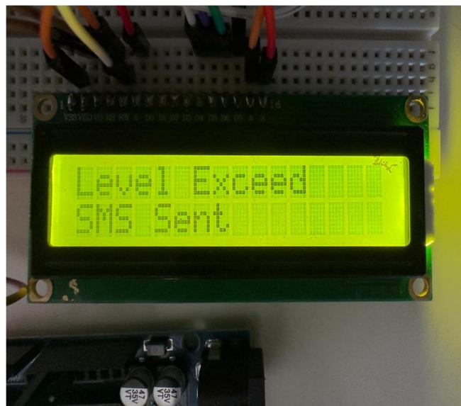
Fig 5: When alcohol level exceeds the threshold
