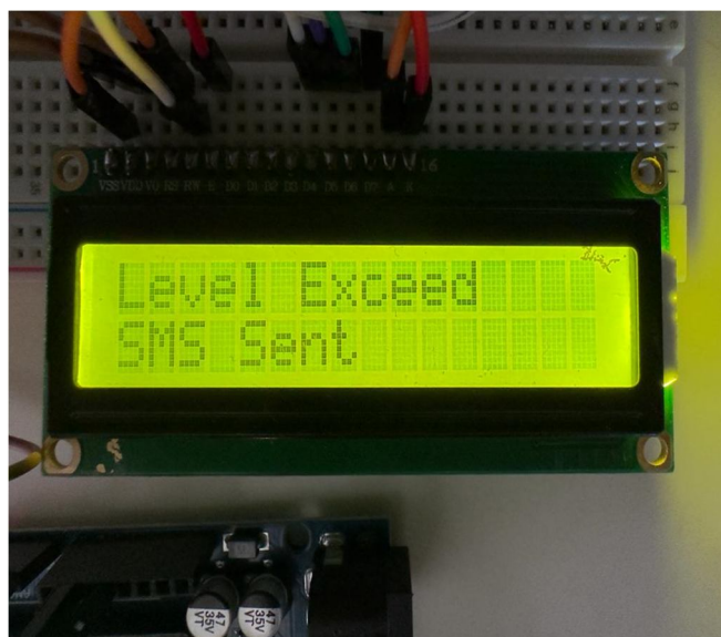
Fig 5: When alcohol level exceeds the threshold
