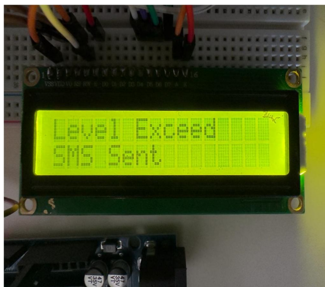
Fig 5: When alcohol level exceeds the threshold
