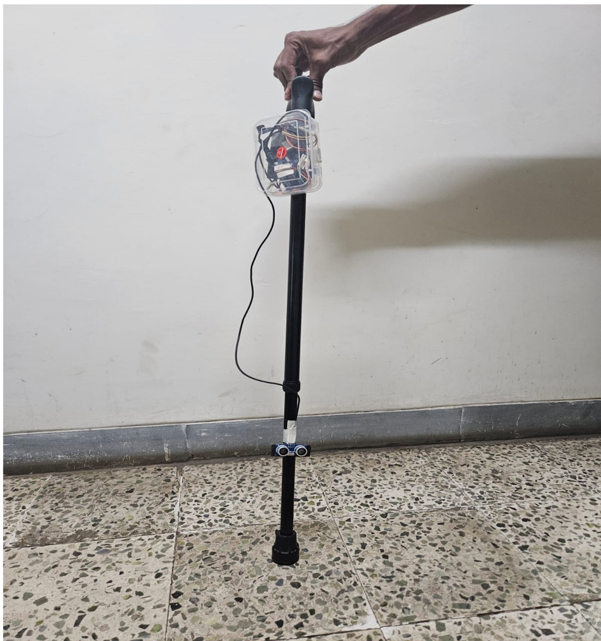
a) Blind stick with complete equipment
