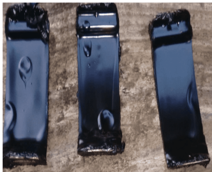
Fig 6. Images of the coupons with the paraffin deposition using 3 kg of crude oil
