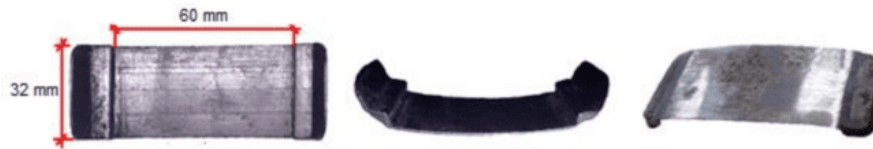
Fig. 2 Images of coupons developed for the paraffin deposition thickness measurement method.
