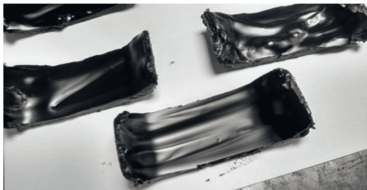
Fig 7. Images of the coupons with the paraffin deposition using 5 kg of crude oil
