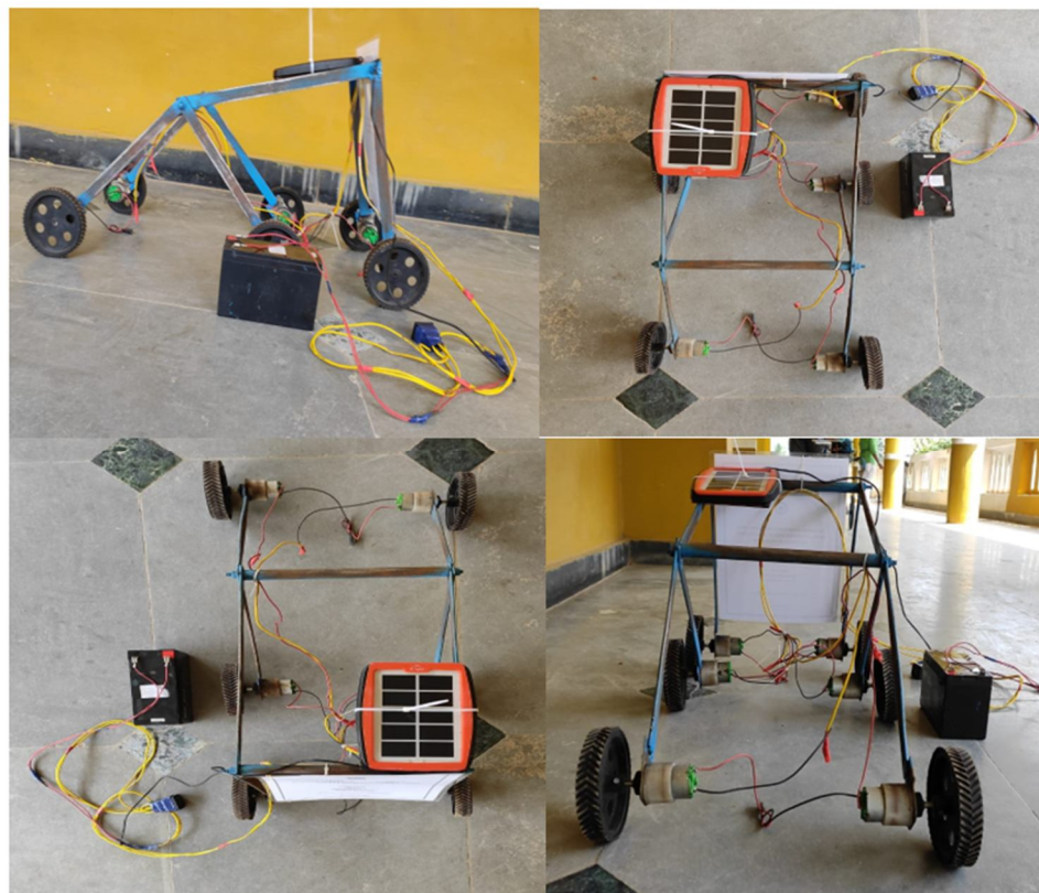
Figure 8. Terrain Vehicle under rocker bogie mechanism
