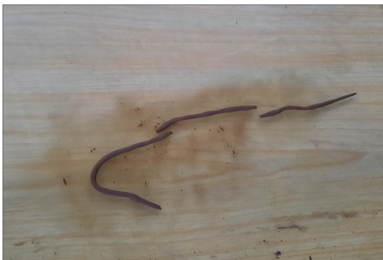
Determination of Plastic limit
