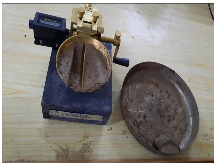
Determination of Liquid limit
