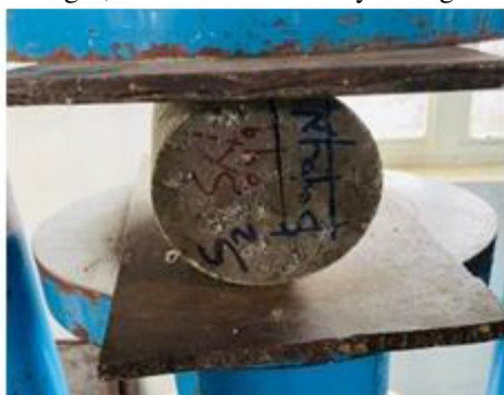
Fig5. Split tensile test
