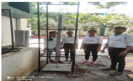
Impact Testing by Drop Weight Hammer
