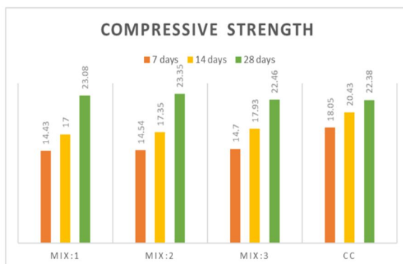
Fig No 6.1 Bar chart of compressive test of cubes using Sea Shell with TiO 2
