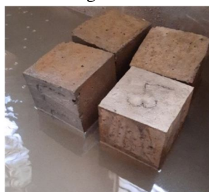
Fig:6 Curing Of Cube
