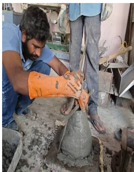
Figure 5 Performing Slump Cone Test
