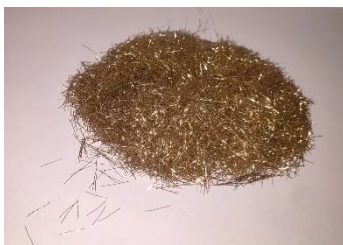
Fig 4: Brass coated Steel Fibres
