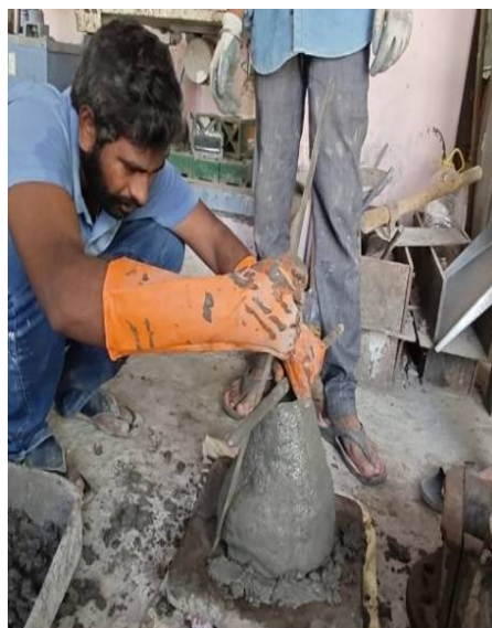
Figure 5 Performing Slump Cone Test
