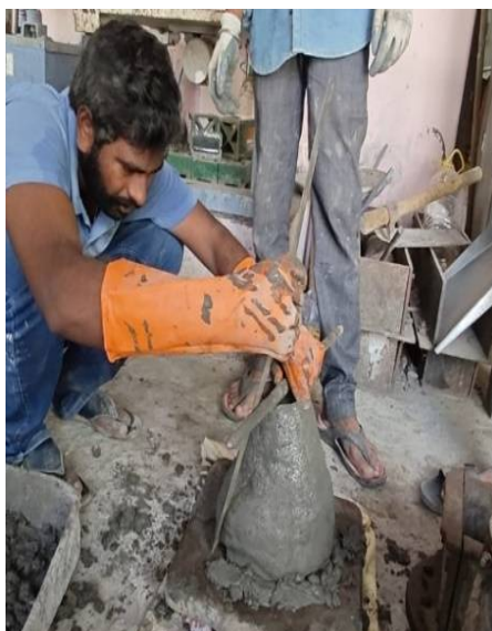
Figure 5 Performing Slump Cone Test
