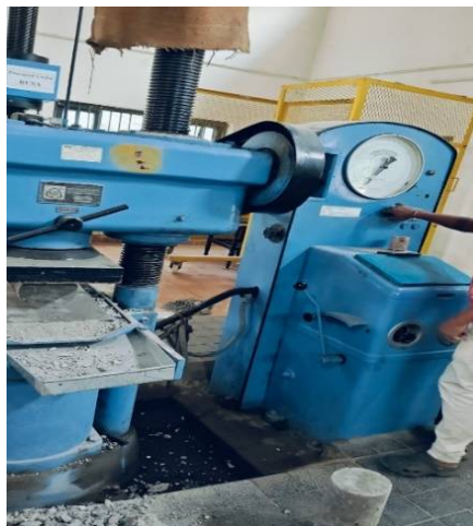
Fig 7. Split Tensile Strength Test
