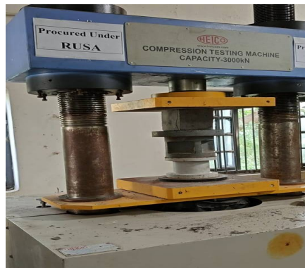
Figure 6. Performing Compressive strength test
