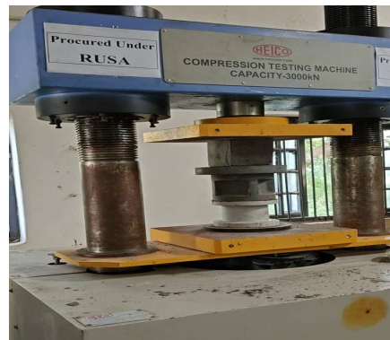
Figure 6. Performing Compressive strength test
