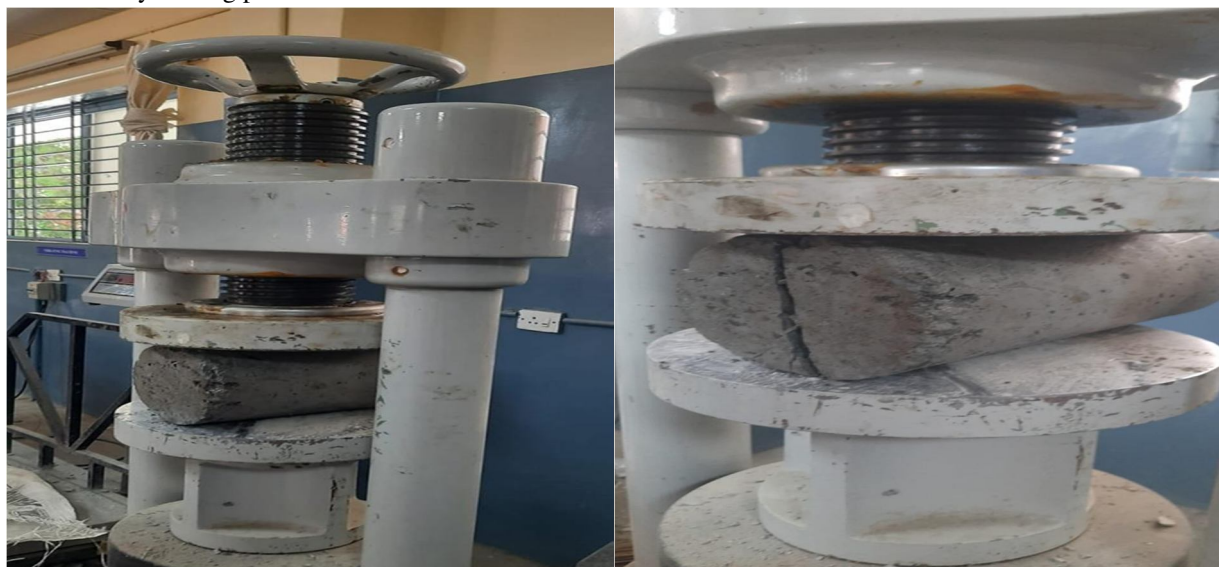
Fig 9: Split tensile strength test
