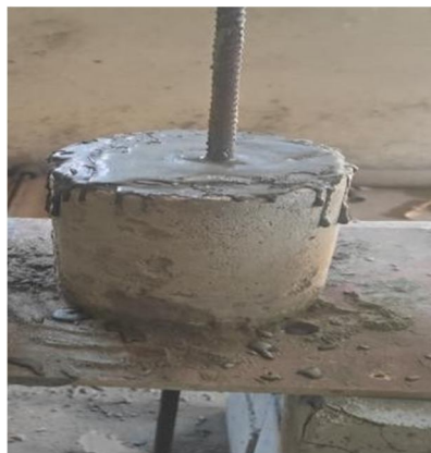
Figure 7 Grouting reinforcing bar into the cylinder
