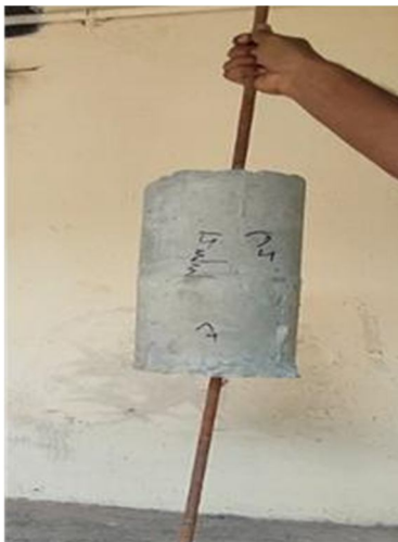
Figure 16 specimen with dowel joint for 12mm with straight and helical end rebar named as S8
