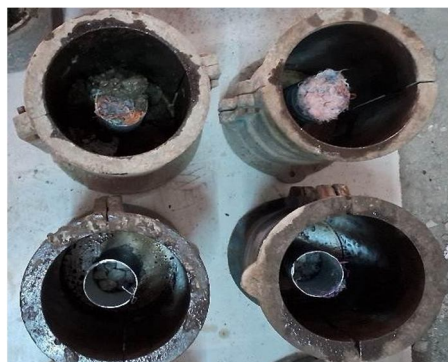
Figure 4 Mould for casting the specimen Figure 5 Hollow cylinder after curing
