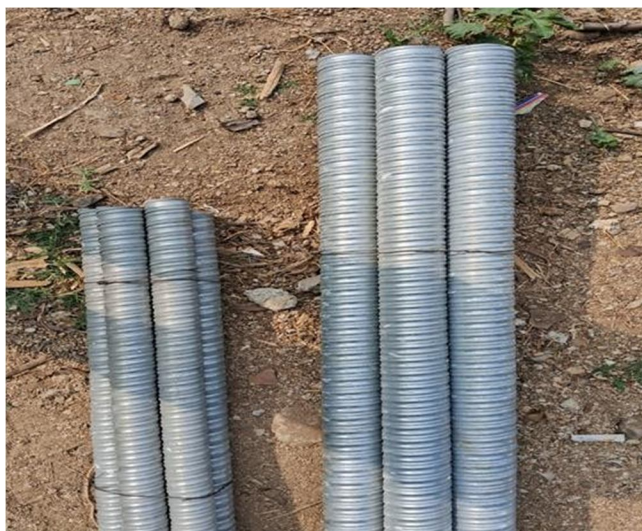
Figure 3 Sleeve of diameter 40mm and 60mm
