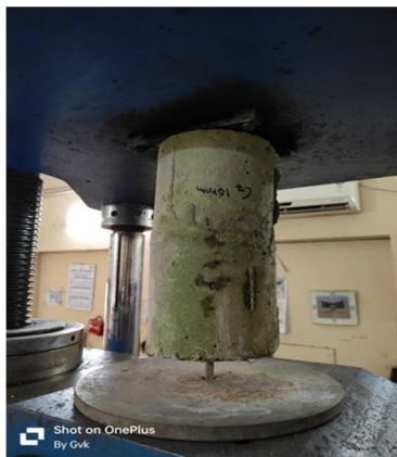
Figure 13 specimen with dowel joint for 10mm with two straight bars named as S3
