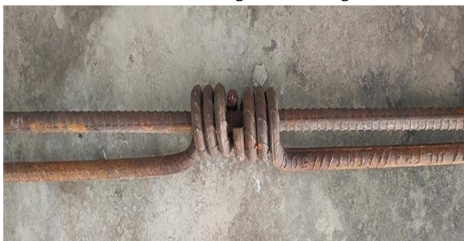
Figure 1 Interlocking of two helical end and a straight rebar for 10mm
