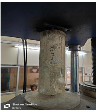
Figure 14 specimen with dowel joint for 12mm with two straight bars named as S7
