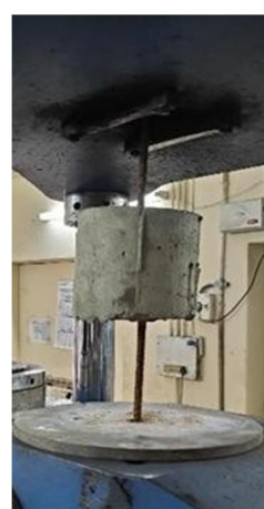
Figure 11 specimen single cylinder with straight bar and helical end of 10mm bars overlapped named as S2
