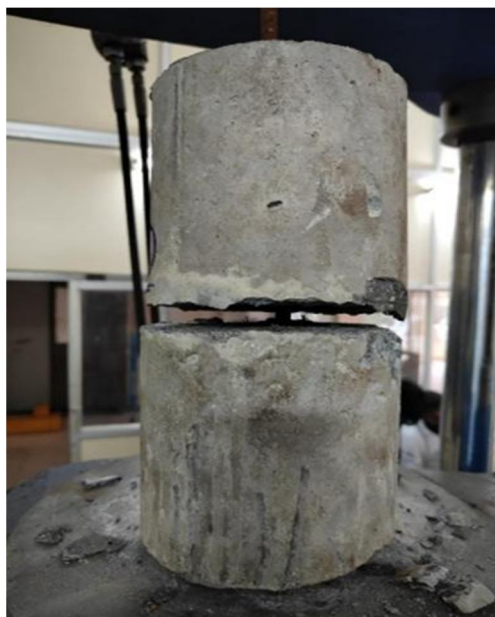
Figure 23 Failure of dowel joint for specimen S4
