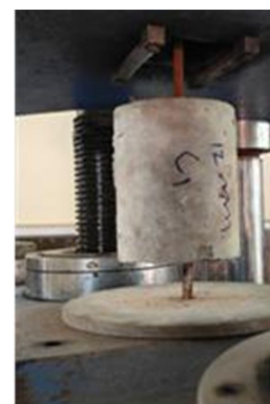
Figure 12 specimen single cylinder with straight bar and helical end of 12mm bars overlapped named as S6
