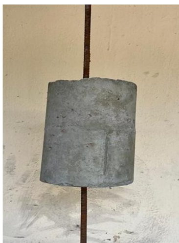
Figure 15 specimen with dowel joint for 10mm with straight and helical end rebar named as S4
