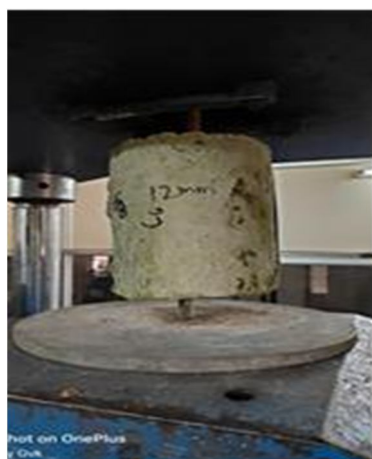
Figure 10 specimen single cylinder with two straight bars of 12mm overlapped named as S5
