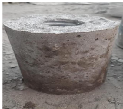
Figure 4 Mould for casting the specimen Figure 5 Hollow cylinder after curing
