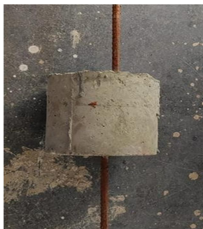
Figure 9 specimen single cylinder with two straight bars of 10mm overlapped named as S1
