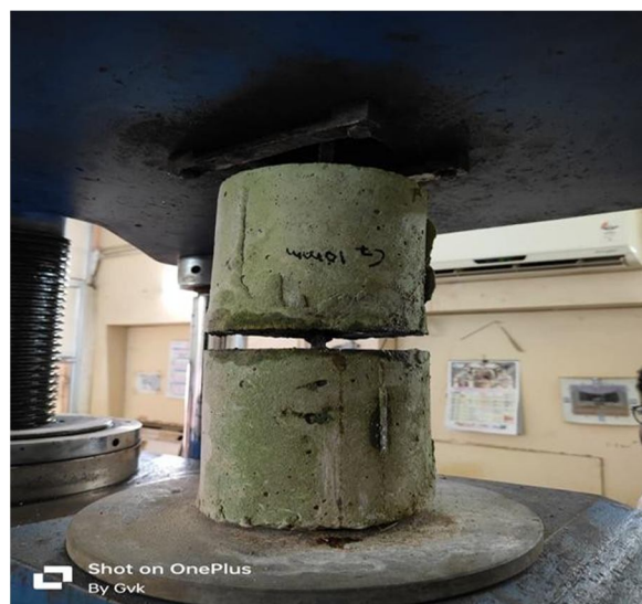
Figure 21 Failure of dowel joint for specimen S3
