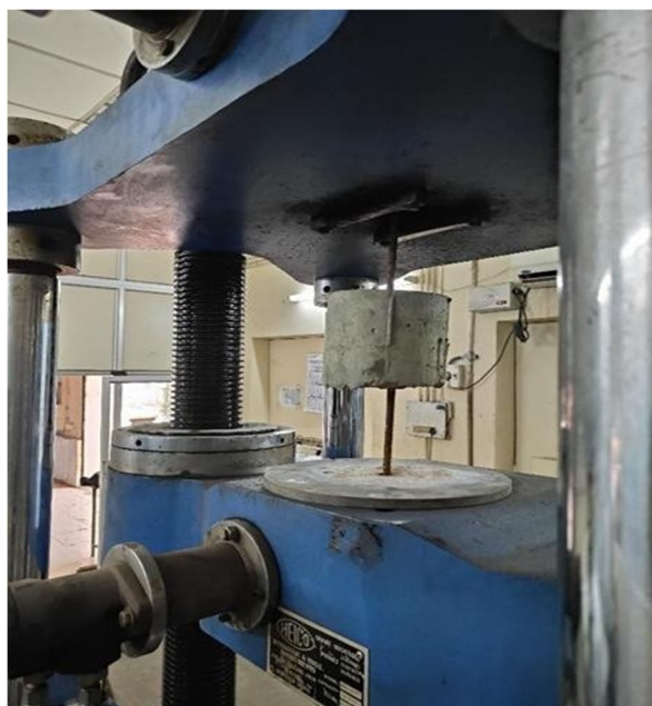
Figure 17 Universal Testing Machine setup with specimen S1
