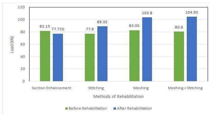
Figure 9.1: Variation of Load of beams BR and AR
