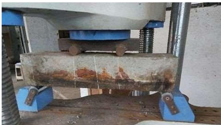
Figure 8.2: Testing of corroded beam before rehabilitation
