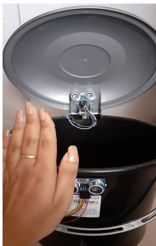
Fig. 11 Lid opens up when object approaches the bin
