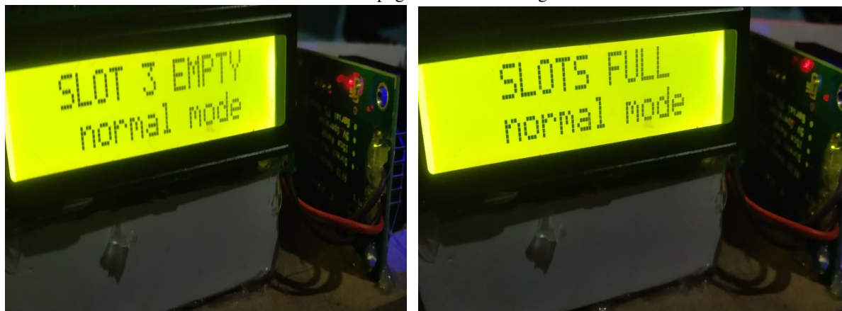
Fig.12; Parking Slot status on LCD showing empty and full in normal mode
