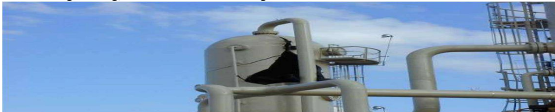
Fig. 2. Failure of pressure vessel during hydro Test.
