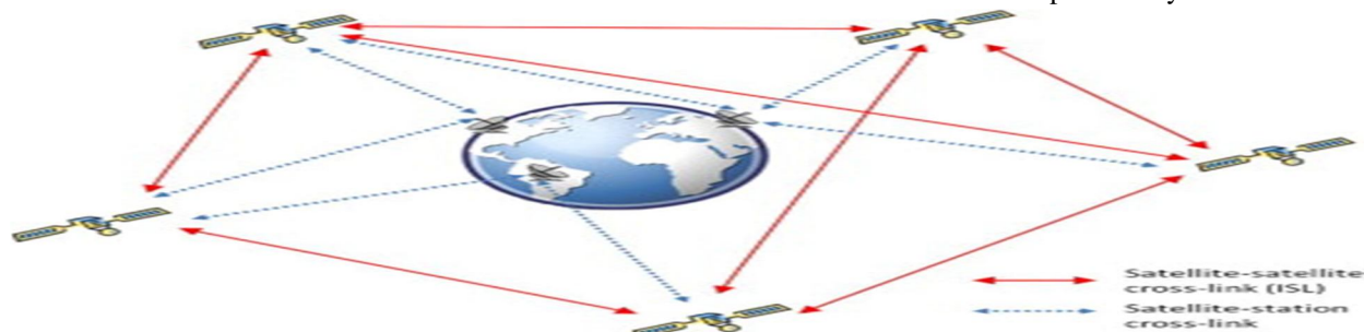
Fig.5 Inter-satellite communication and satellite-station communication
