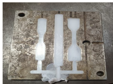
Figure 7. HDPE injection molding specimen in die
