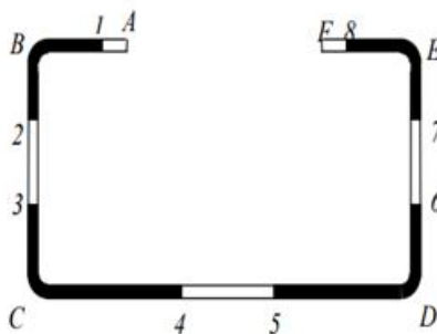
Fig. 9 Effective widths of compression elements
