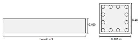
Figure 7: Design of Column ( 5-8 floor)
