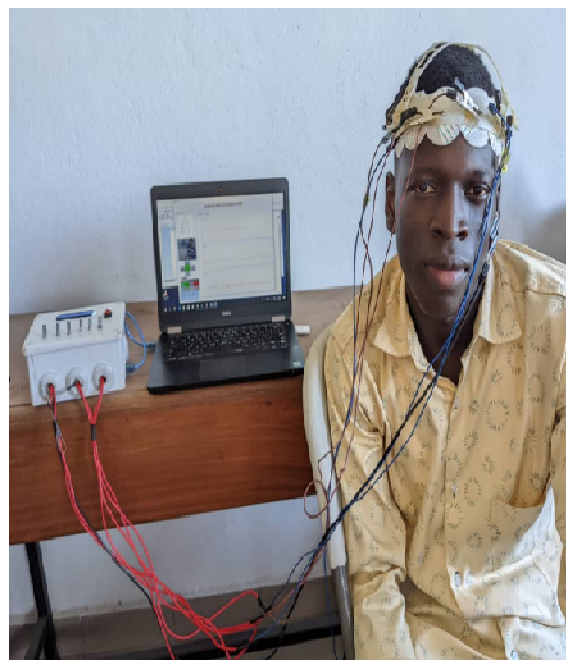
Fig.2. Patientdata collection deviceinstalled
