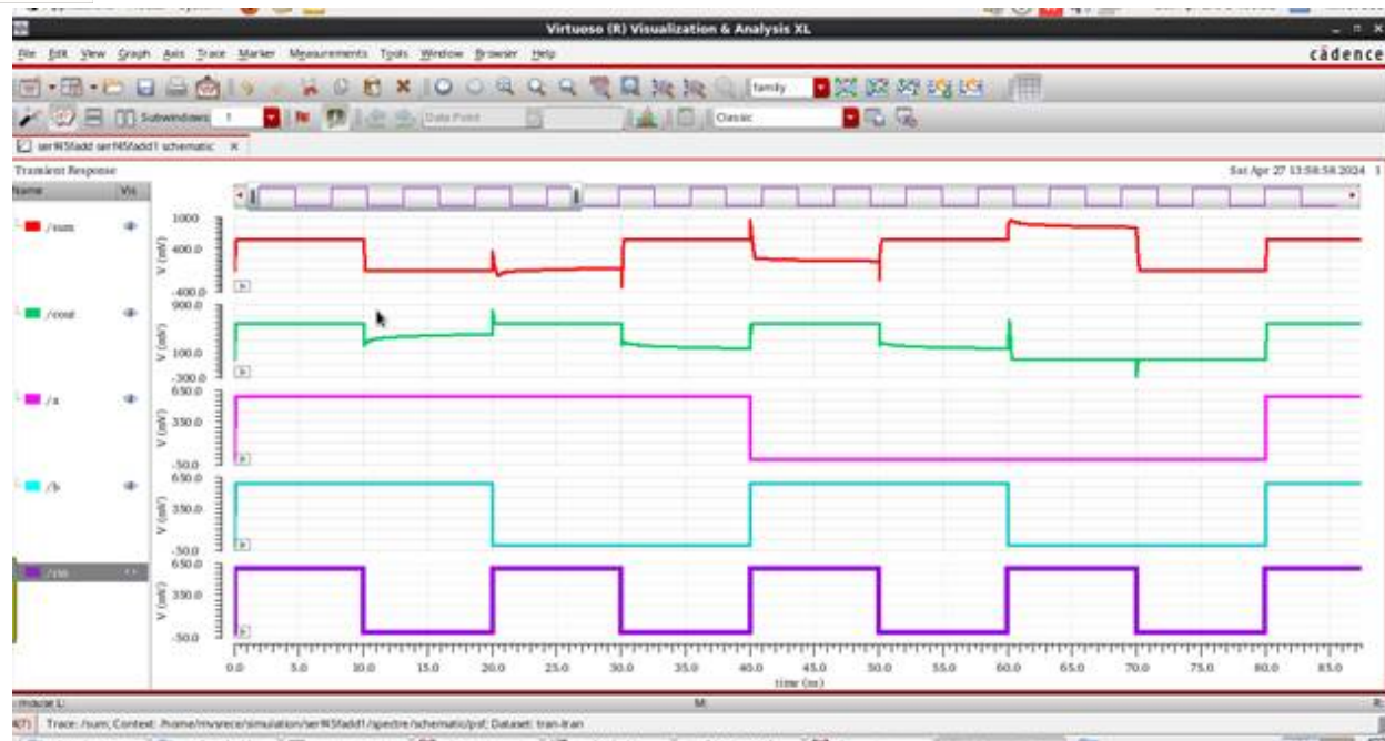
Fig. 8 Output of 10T SERF full adder
