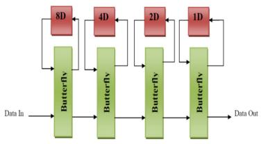
It has single butterfly processor for performing signed addition and signed subtraction function. Single path delay elements have been used in the feedback structure.
