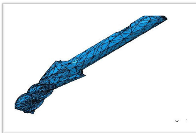
Fig. 7 Static case solution-Deformed mesh
