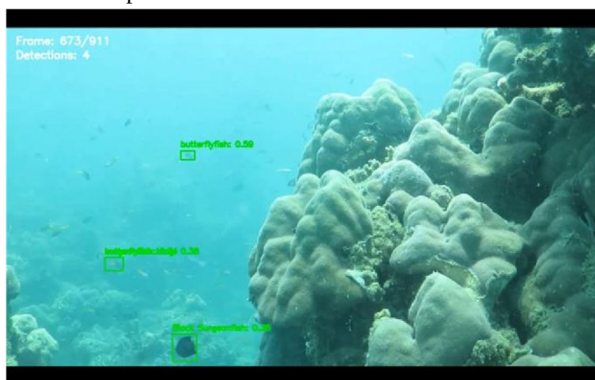
Fig. 6. Representative SSD300 detection output on an underwater fish image.
