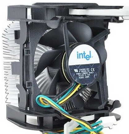
Fig. Exhaust fan with Aluminum heat sink
