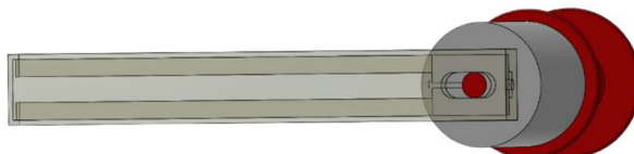
Fig.14 Transparent view of the swingarm attached to the wheel hub
