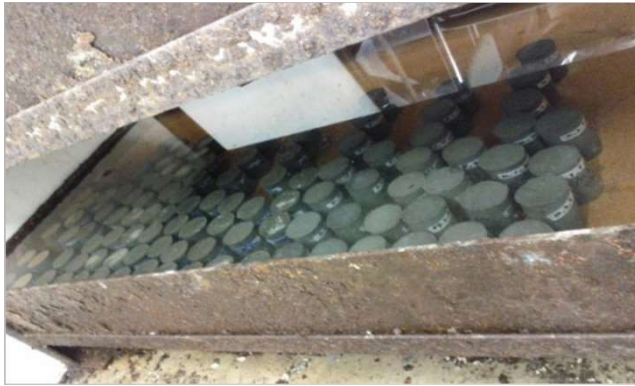
Fig. Concrete cylinders curing in lime saturated water
