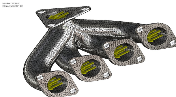
Fig. 4 Exhaust gallery meshing
