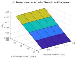
showing a clear trend that lift increases with stronger actuation and is maximised when the actuator is placed near the leading edge. (See Appendix C for code used.)
