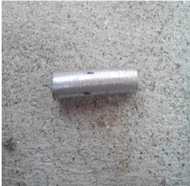
Fig. 3.7 Wear test specimen
