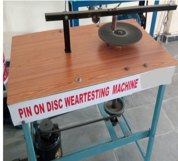
Fig3.8 Pinon disc wear testing equipment
