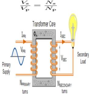
By appropriate selection of the ratio of turns, a transformer thus enables an alternating current (AC) voltage to be "stepped up" by making Ns greater than Np, or "stepped down" by making Ns less than Np.
