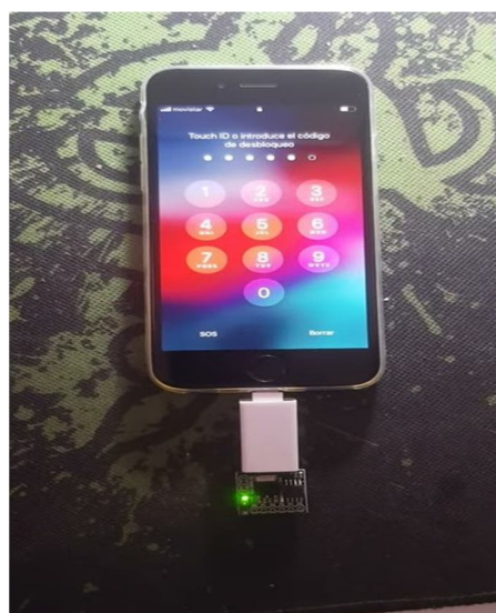
Fig.7.Connecting ATtiny 85 to mobile
