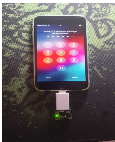
Fig.7.Connecting ATtiny 85 to mobile
