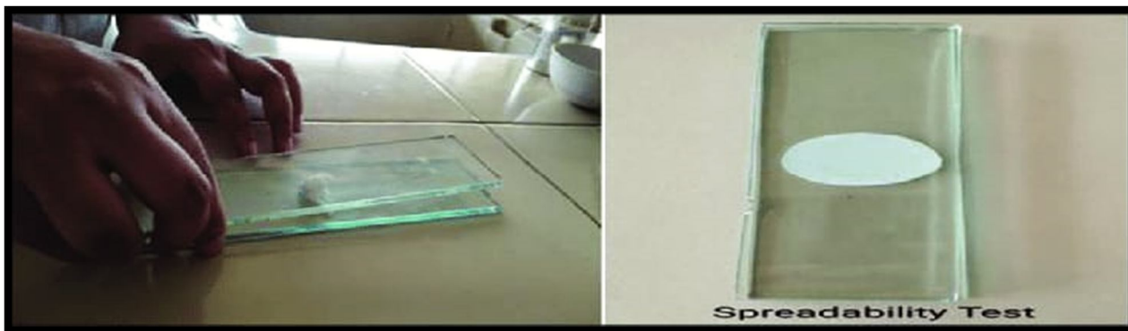
Fig No (8) :- Spreadability test
