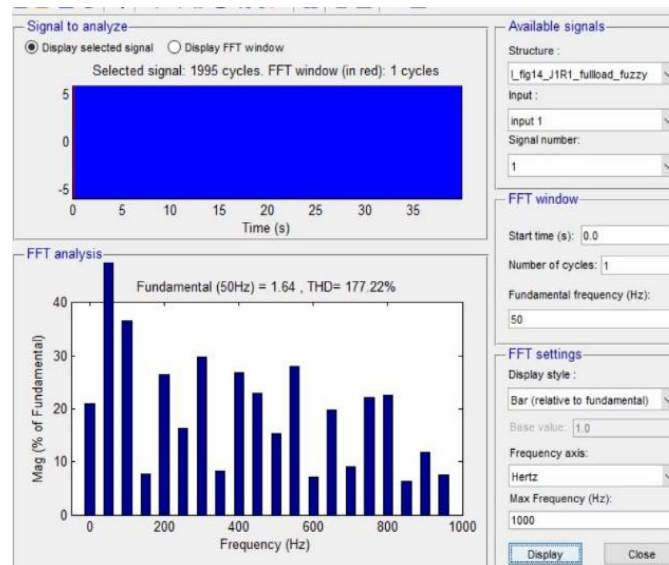
Fig. 17. Fuzzy PID controller response of J1 &amp; R1 with full load
