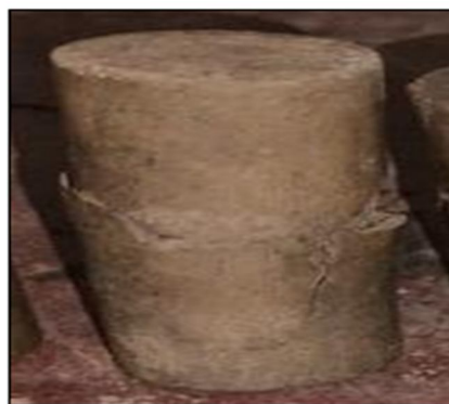
UCS SAMPLE FAILURE PATTERN
