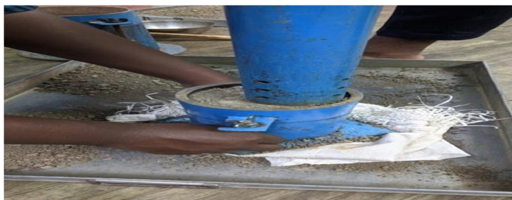
Modified proctor test (Heavy compaction)
