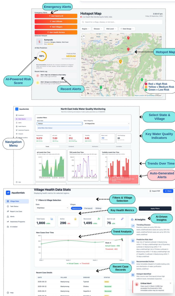
Fig. 8. Health official web dashboard: (a) geo-tagged hotspot map, (b) village health data statistics, (c) AI-driven prediction panel.
