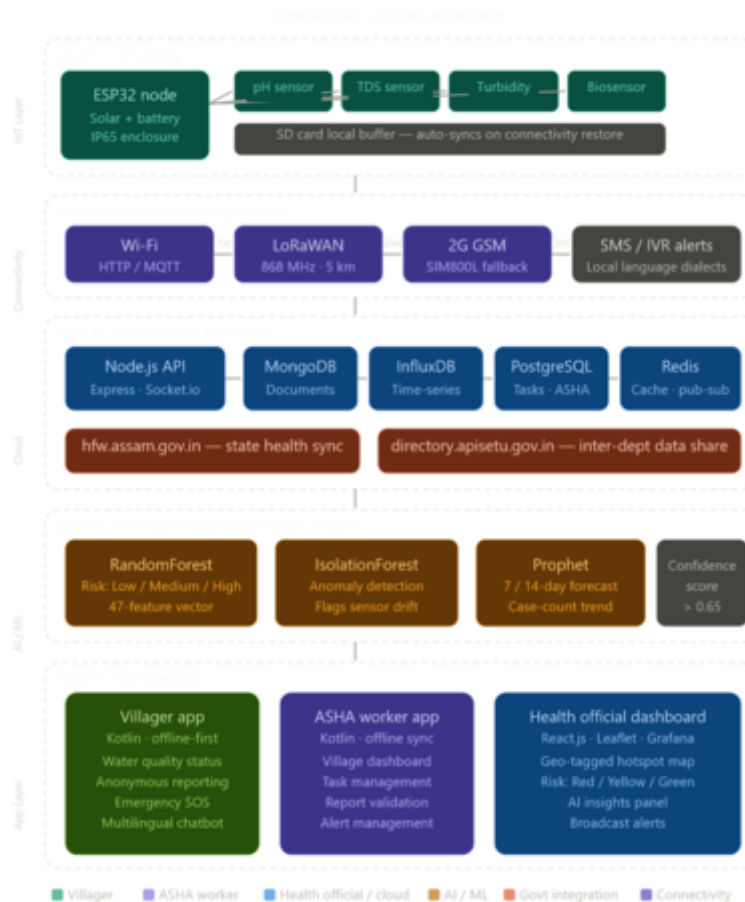
Fig. 2. High-level AquaSentials system architecture showing data flow from IoT sensors through cloud backend to user dashboards.
