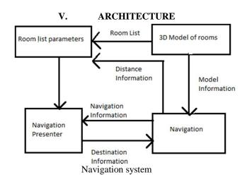
The structure has mainly two portions, that are the navigation part and a section containing room list and 3D models. The 3D models are built with the parameters extracted from the map of the building, which is used to create a list of rooms to provide in the menu displayed in UI. This information is passed on to the navigation section where we are building virtual environment matching to the real world
