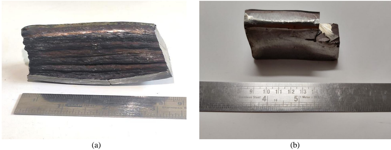
Figure 5. (a) Unpolished block after additive manufacturing (b) Polished Block
