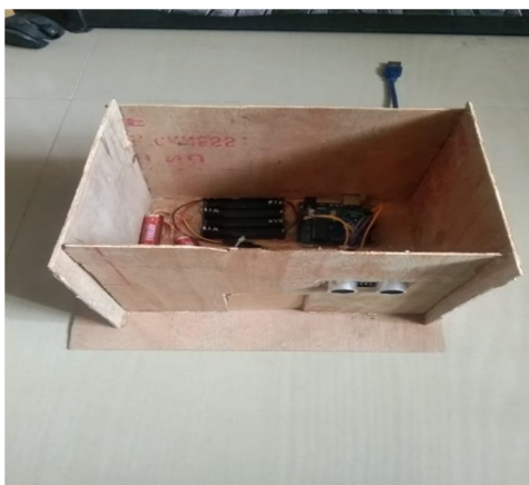
Fig2 : A compact prototype setup consisting of an Arduino microcontroller, battery pack, and connected electronic components arranged inside a wooden enclosure. The system is powered via a USB cable and demonstrates the basic hardware integration of the projec
